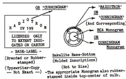
The first "UX" tubes were released about mid-1925. Base-label style #1 (see page 3) was used. The RCA (but not the Cunningham) monogram and the 'License Clause' were molded on the bottom of the tube-base. The RCA (or Cunningham) Monogram was rubber-stamped inside the top center of the bulb where possible, or on the side of the bulb. These features were standard for the UX- and UY-tubes until early 1928.
