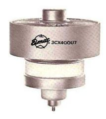
200 watts of useful CW rf power may be obtained with better than 33% efficiency, and better than 10 dB of gain. At frequencies near 900 MHz the amplifier circuit may be essentially a quarter-wave radial or rectangular resonator for the anode, and a three-quarter wave coaxial line section between ground and cathode. The amplifier is described in this data sheet. Terminal collets are available and are listed.
